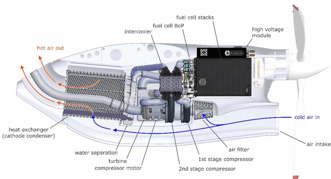
*Figure 3 - Conceptual integration of an IE-FLIGHT F300 fuel cell product in a future fixed wing propulsion system*
