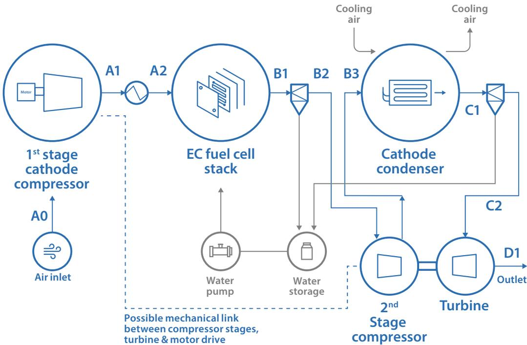
Figure 4 - Comparison of conventional EC and EC HT architecture
