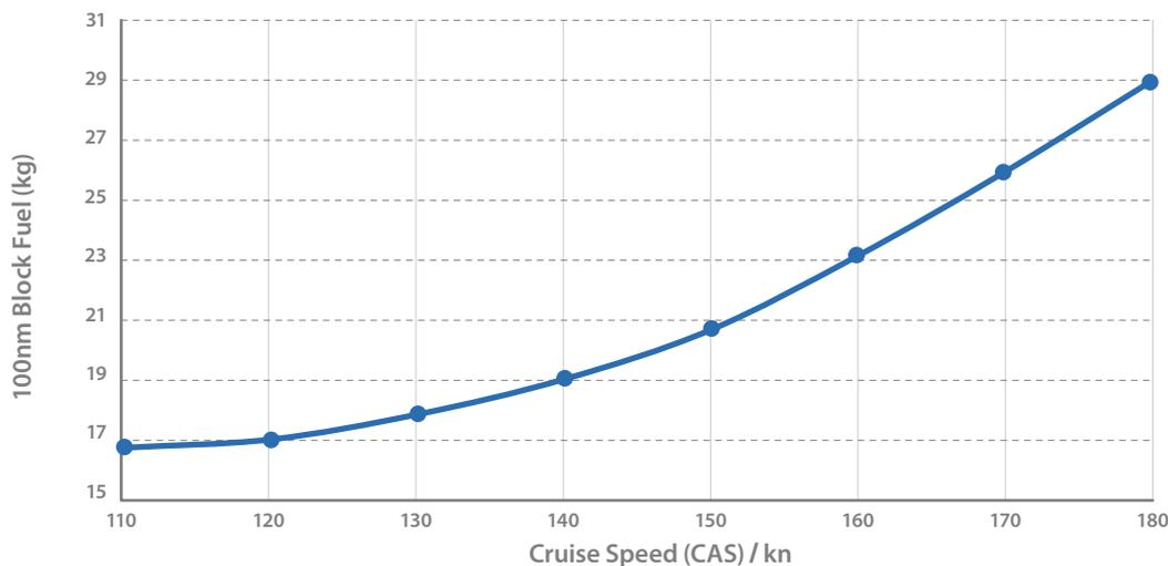
Figure 6 - Comparison of cruise speed against block fuel
