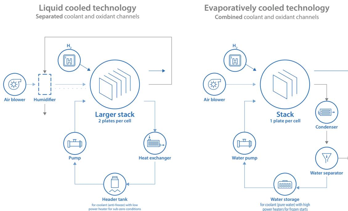
Figure 1 Comparison of Liquid Cooled and Evaporatively Cooled Fuel Cell Technology
