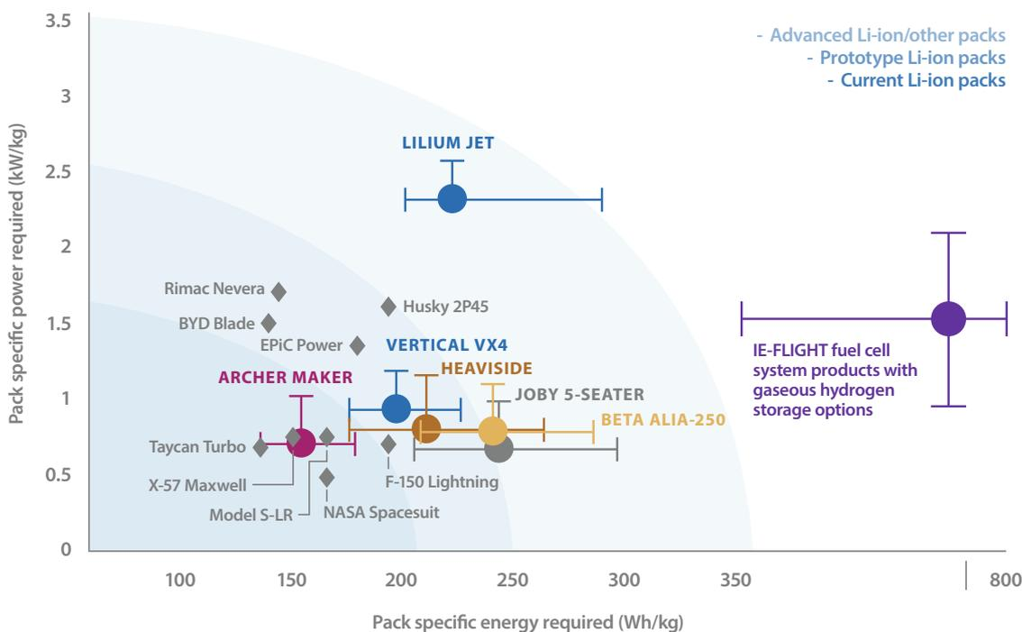
*Figure 8 - Carnegie Mellon study on battery technology performance, eVTOL manufacturer battery requirements to meet their range requirements, and IE-FLIGHT™ fuel cell system performance.*
