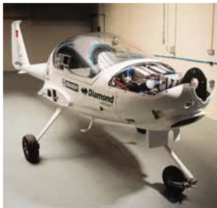
Integrated 20kW fuel cell system
